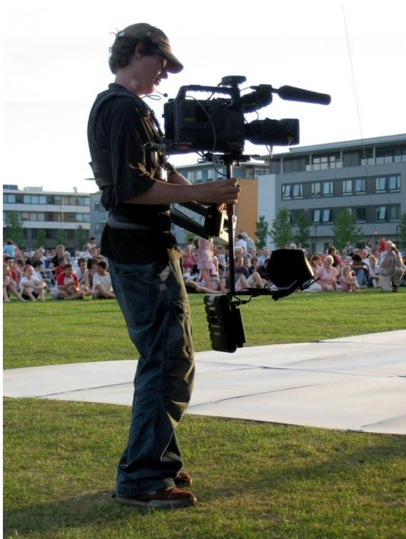
The spring suspension operates at a mechanical *dis*advantage so that changes in the relative height of the operators harness relative to the camera made insignificant changes to the spring length and therefore the vertical force remains as the weight of the camera assembly. The suspension has high compliance. The operator uses his hands to make adjustments to the camera height and direction, and once made these need not be changed.
